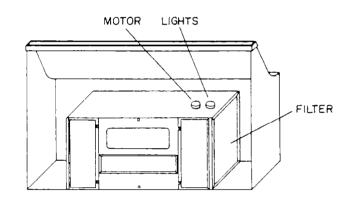
For most efficient smoke removal, the top of the hood should be approximately 66 inches (167.6 cm) from the floor.
